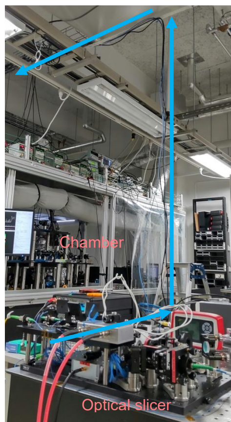
Fig. 1 Photograph of the optical slicer. The optical pulses are sent to the chamber (back) through a fiber.
