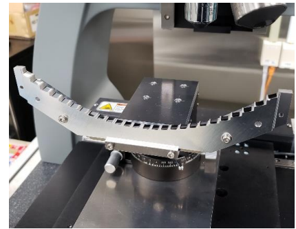
Fig 3 Test product of the pupil-mirror array.
