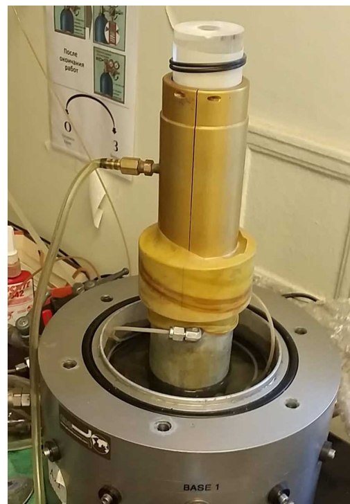
Fig. 4: Placing sample in the Triaxial Machine for testing
