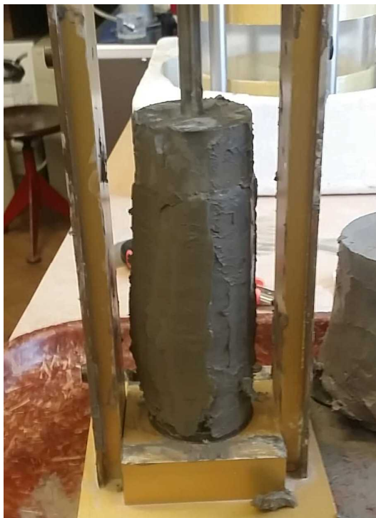
Fig. 3: Trimming sample according the mold dimensions
