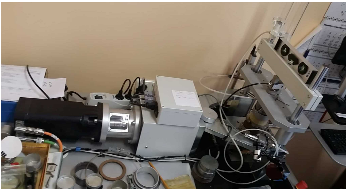
Fig. 7: Ring Shear Test Apparatus for testing Martian Soil
