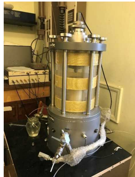
Fig e: Specimen during saturation
