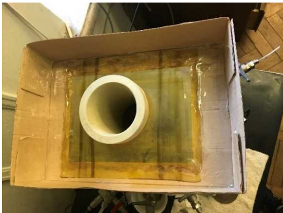
Fig d: Mold for pluviation of sample
