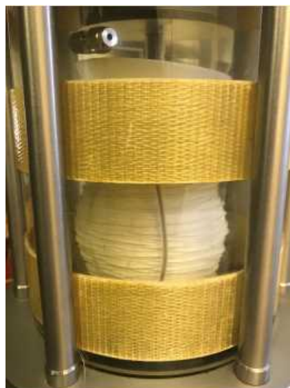
Fig d: Mold for pluviation of sample
