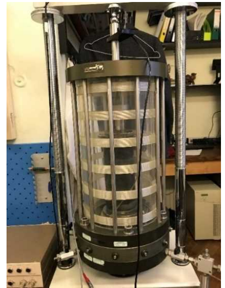
Fig c : Triaxial Apparatus with undisturbed sample
