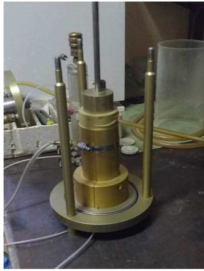
Fig. 2 Placing of top cap
