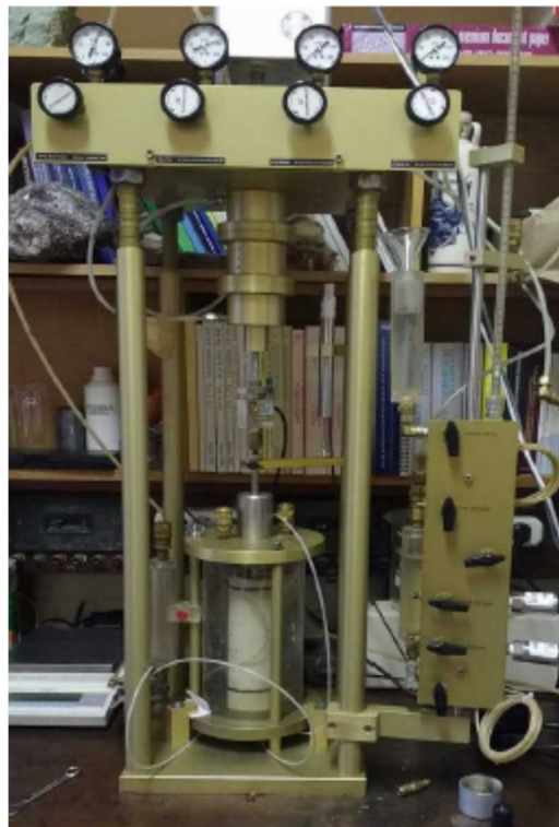
Fig. 4 Assembly for triaxial testing
