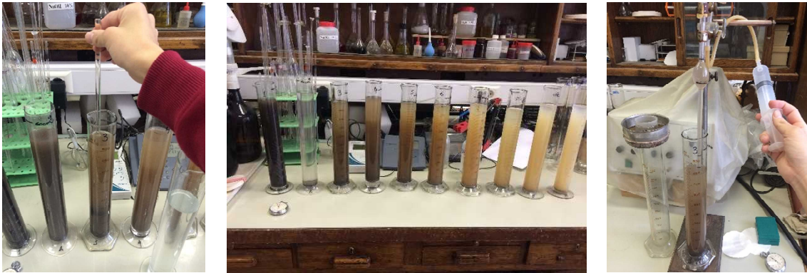
Fig.2 The process of cylinder method (Mixing- Waiting for settlement- Sampling)
