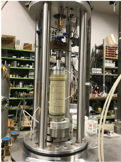
Fig.1. Triaxial tests for coarse sand (a); triaxial tests for gravel (b)
