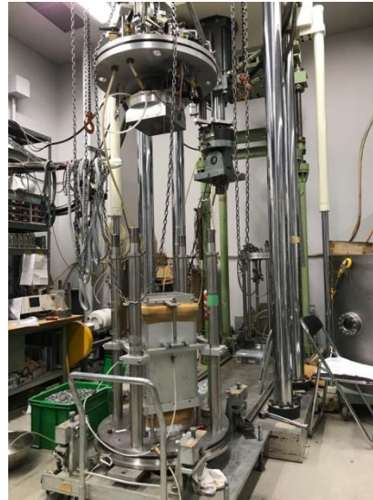
Fig.1. Triaxial tests for coarse sand (a); triaxial tests for gravel (b)
