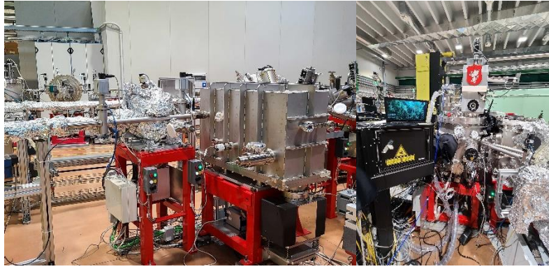
Figure. Photos of the optical setup for soft X-ray SFG we constructed at EIS-TIMER beamline at FERMI, taken at (left) the upstream and (right) the downstream of the XFEL beam.
