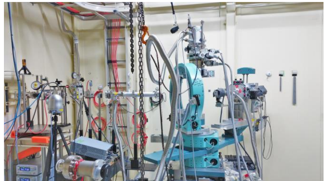
Fig. 1. Inside view of the experimental hatch. Green equipment is the 4-cycle diffractometer and helium refrigerator is mounted on top of it. The sample is in the refrigerator.
