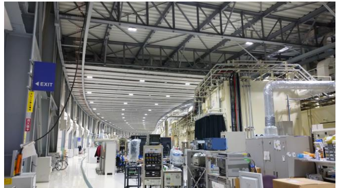
Fig. 2. Experimental hall of SPring-8. In SPring-8, electrons are accelerated and stored in a ring with a circumference of 1,400 meters. X rays are emitted from the electrons and guided to each beam line and experimental hatch (right side of the figure). Experimental equipment is remotely controlled from the outside.
