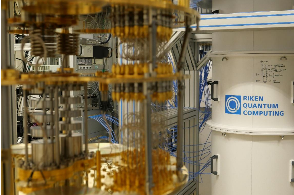
Figure 1. A dilution fridge used for superconducting qubit experiments.
