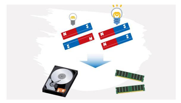
In laptops, hard disk drives (HDD) are a common device for secondary storage. Basically, HDD consist of several platters or disks, Read-and-Write heads and arms. A binary data is physically processed in the form of a configuration of numerous small magnetic domains or their boundaries. This corresponds to a situation where many bar magnets are arranged on the disk.
