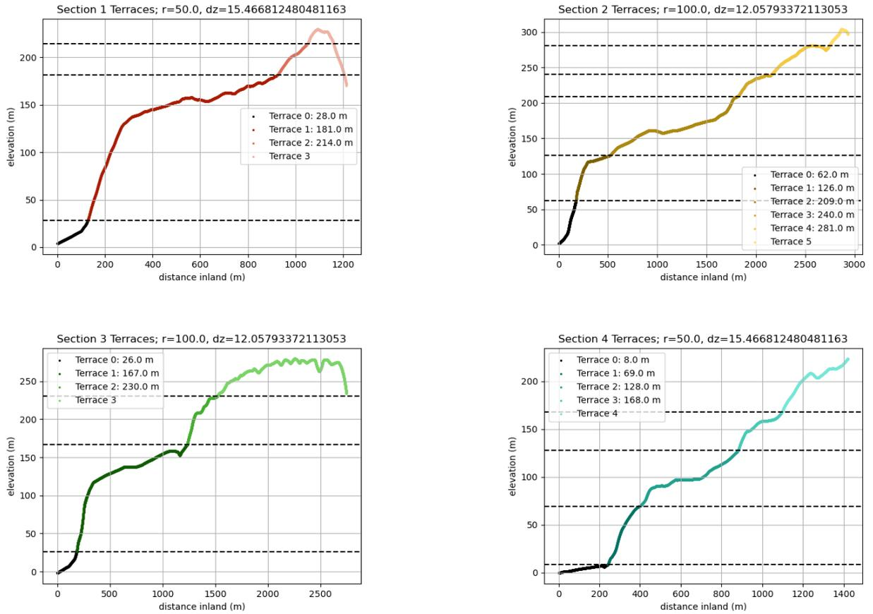
Figure 3: Identified terrace inner edges in Sections 1-4 from Figure 1. Terrace 0 in all graphs represents the transition from beach to terrace formations (limited diagnostic accuracy, as seen in Section 2). Comparison between inner edges and previous literature can be found in Table 1.
