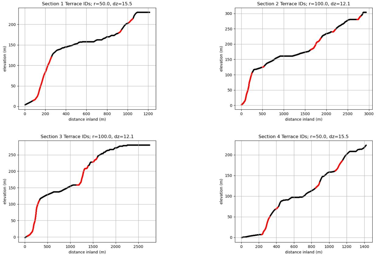
Figure 2: Vertical cross-sections of Sections 1-4 from Figure 1 partway through terrace inner edge identification. A smoothing function has been applied to the true cross-sections to create monotonically increasing geometry, and highlighted in red are areas identified with sufficient increase to satisfy Equation 1.
