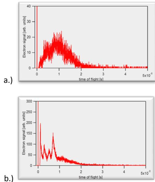
**Figure 2.** Photoelectron Spectrum of He gas using Neon HHG. a.) Spectrum before addition of focusing mirror. b.) Spectrum after addition and adjustment of focusing mirror.
