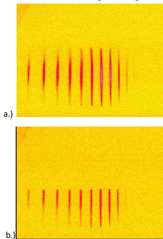
**Figure1.** High order Harmonic generation with Neon gas and 800nm light pulsed at 30-40 fs. a.) HHG spectrum without Aluminum filter b.) HHG spectrum with Aluminum filter of transmission >17.42nm
