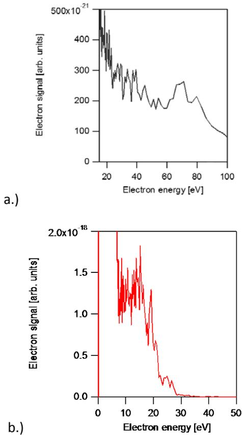
**Figure 6.** Photoelectron energy spectra of He corresponding to Figure 3. A.) Using Neon HHG. b.) Using Argon HHG
