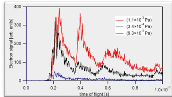
**Figure 4.** Photoelectron spectrum of Helium using Ar HHG at varying Helium gas pressures. Magnetic fields were kept constant at 950mT and 2.1mT.
