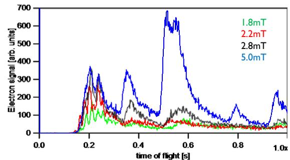
**Figure 5.** Photoelectron spectra of He using Ar HHG at varying flight tube magnetic fields,  $B_f$  while  $B_i$  is held at approximately 960mT. Sample gas pressure for all spectra was  $1.7 \times 10^{-3}$  Pa
