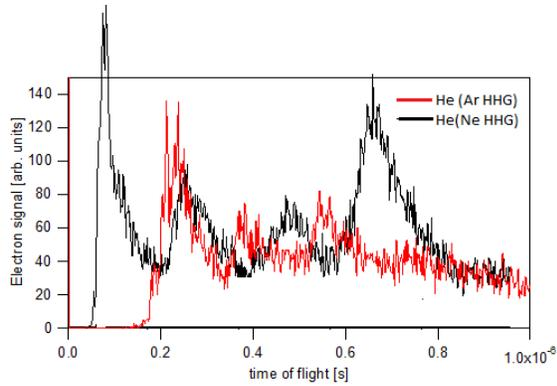
**Figure 3.** Photoelectron spectra of He using Ar HHG (red) and Neon HHG (black). Both spectra were taken at approximately  $3 \times 10^{-3}$  Pa with magnetic fields at 900mT, and 3.8mT.
