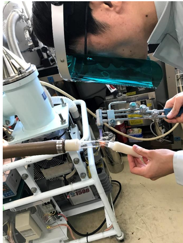
Sealing of the quartz tube while evacuating the sample space with a diffusion pump.
