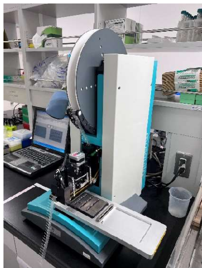
Figure (A) The mosquito crystal robot for mixing the RNA solution and reservoir solution together to make a sitting drop for crystallization. (B) The microscope to observe the crystallization condition and (C) the crystal of magnesium phosphate I found in my condition screening.
